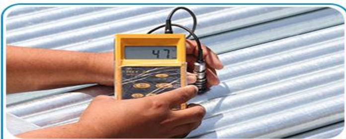
Zinc Coating Test
